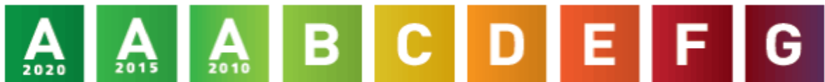
Figure 8 The EPC scale, the scale goes from A to G, where A is the best label, A2020 is reserved for new buildings.
