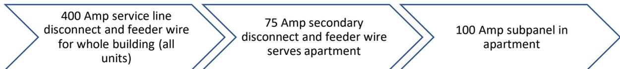
**Figure 25. Electrical Infrastructure Assumptions for Example Calculation**
