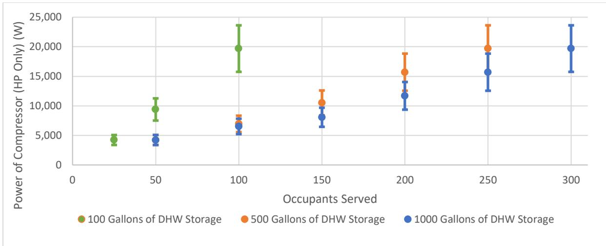
**Figure 31. Central HPWH Power Consumption Data**
