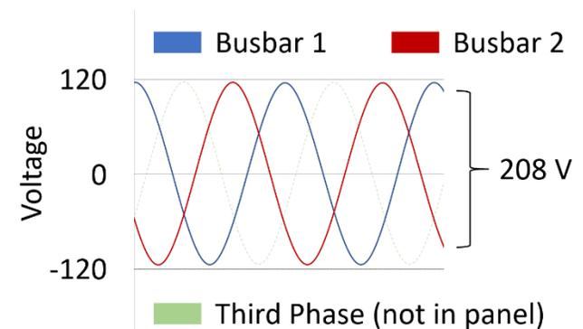
**Figure 5 Three-Phase Power**
