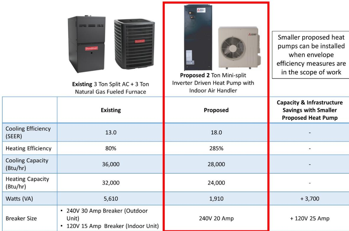
**Figure 30. 1.5 to 3 Ton Split AC Replaced with Heat Pump with Efficiency Measures Applied**
