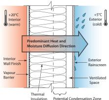
An air barrier system should be continuous around all components of the building, with special attention given to walls, roof and the lowest floor. There must be proper continuity at intersections, such as the connection between floors, the joints between walls and windows or doors, and the joint between walls and the roof.
