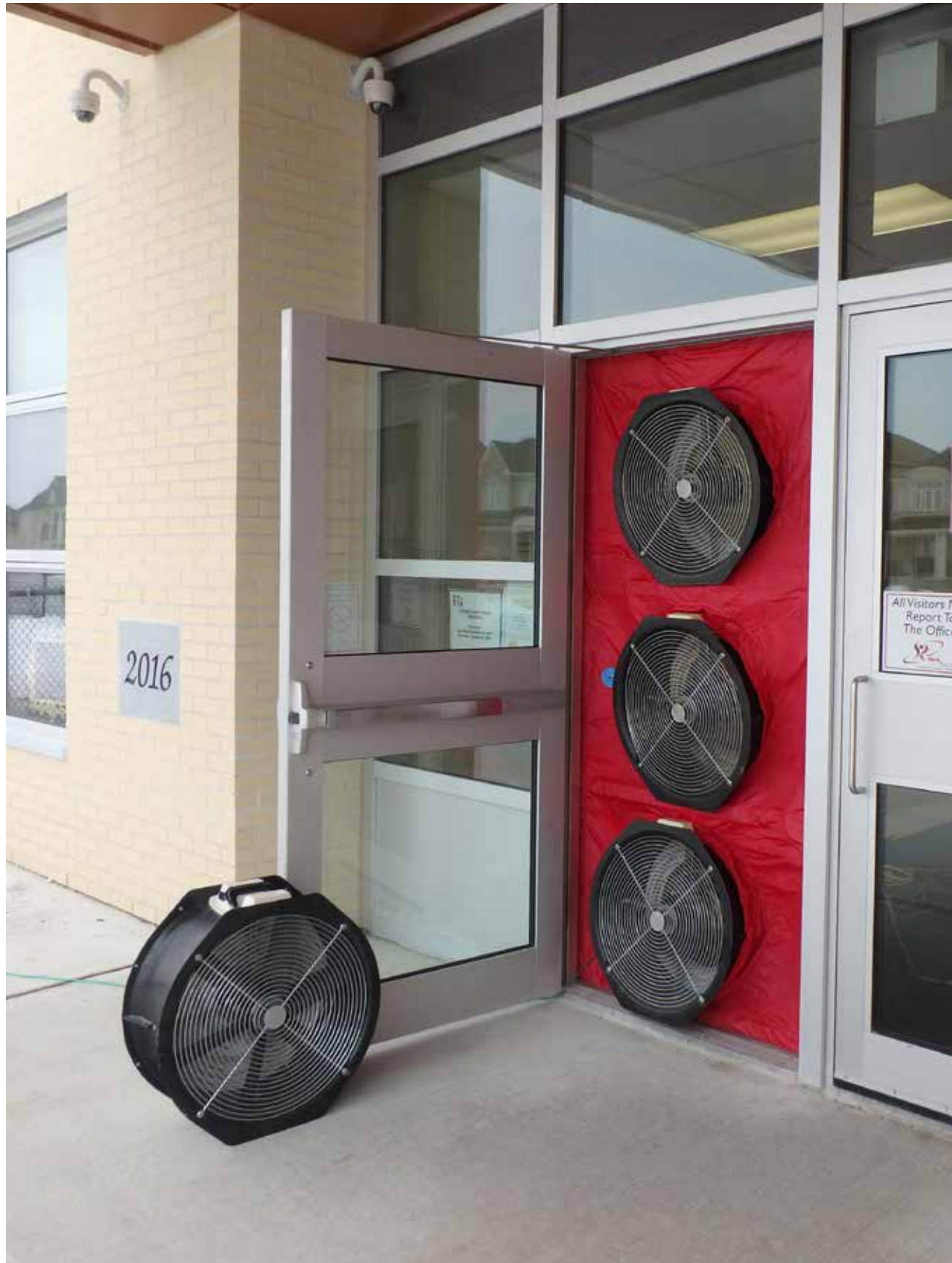
Multiple high-powered blower fans installed in a door opening
